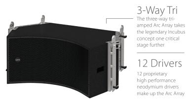
An all-new four-point rigging system with a range of tilt angles from 0° to 10° in five discrete increments makes rigging Arc Array a safe and simple experience for system techs. Housed in a heavily braced 15mm birch plywood enclosure with road proven TourCoat polyurea finish, Arc Array is designed for efficient trucking and handling. Two Neutrik speakON™ NL8s are provided for driver connections.
