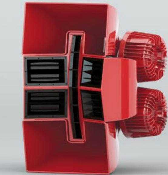
This configuration reduces all forms of destructive interference, maintaining an even frequency response within every degree of the stated coverage angles. Path length compensation devices housed within the waveguides marry with the extended upper response of the compression drivers, allowing the HF to extend up to 26 kHz.
